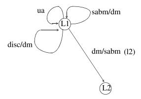
The initialization path (ipl1) which brings the DTE to the Disconnected Phase (state L1) is not shown in this figure. The path ipl1 is given by the Termination Phase part of the specification. It is added as a preamble to the test cases generated for state L1.
