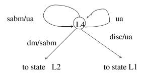
We want to obtain the verification paths for states L1, L2 and L4. Let us start by looking for the potential verification paths of each state. The potential verification paths of state L1, which are obtained from the transition tree of state L1, are:
